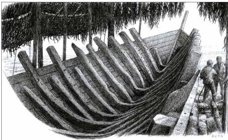
Line drawing, the construction of a hull at Tanah Beru, Richard Gregory. From: Boats in Sulawesi: An illustrated Journey - Australian National Maritime Museum, 19 July 2016 https://www.sea.museum/2016/07/19/boats
