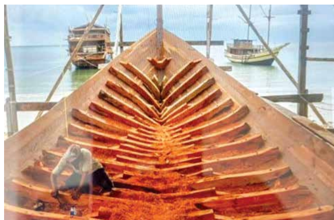
The construction of a pinisi hull. Indonesia's traditional boat builders reach into the past. Agence France Presse, 12 July 2018, au.news.yahoo.com
